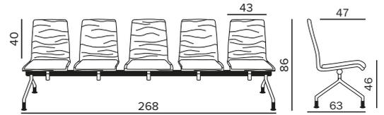
The specified dimensions apply to the wooden shell.
